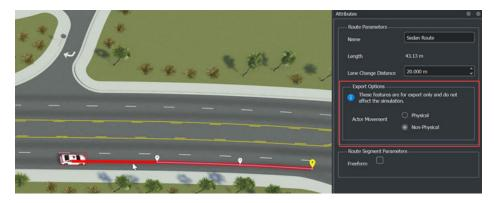
The **Actor Movement** setting does not affect the simulation in RoadRunner Scenario. Physical and non-physical motion attributes on paths affect only files exported to the ASAM OpenSCENARIO format, which you can use in simulators that consider the dynamic constraints of the actor.
