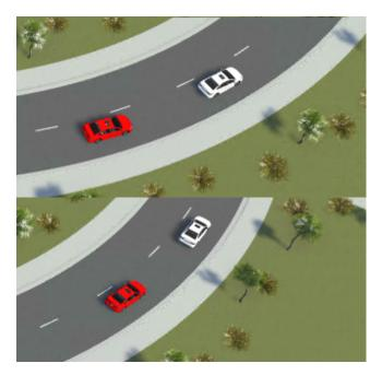
You can now specify the Longitudinal Distance to Actor end condition to action phases in the Logic Editor. Use this condition to end the associated action phase when the actor reaches the specified longitudinal distance from the reference actor.
